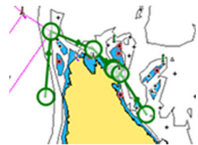
Result after automatic routing
